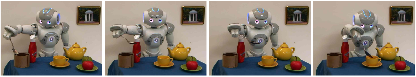
Fig. 7. Execution of DGMP for the powder transfer task. The robot successfully keeps the spoon level while avoiding obstacles not seen in the demonstrations.
