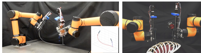
Fig. 1. Two images of the CRISP robot, where 2 manipulators adjust the base poses of needle-diameter tubes that are inserted into the body and assembled into a parallel structure.
