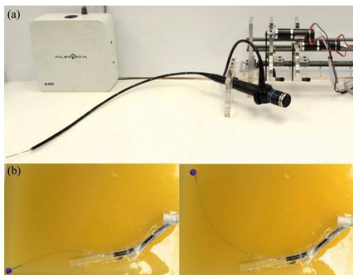
Fig. 3. (a) Our complete system, in which the concentric tube robot and steerable needle pass through the bronchoscope port. (b) Photographs of phantom targeting experiments with the system, in which magnetic tracking feedback was used to steer the needle to targets [3].
